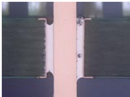
Figure 1. PIP joint without additional solder preform.
