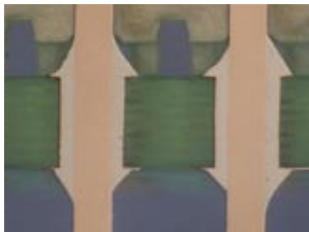
Figure 2. PIP joint with additional solder preform.
