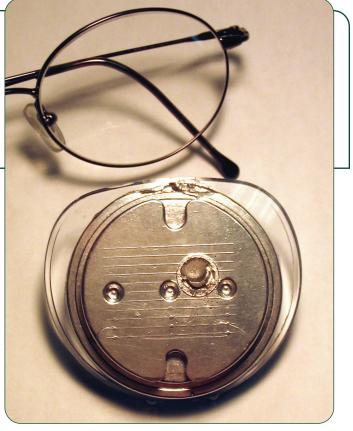
The surfacing block is then mounted in a chuck and is used to protect the lens during the grinding operation. After the grinding operation, plastic lenses are removed from the surfacing block by the inertia of knocking the surfacing block on a solid surface. Glass lenses are removed by dipping them into a hot water bath. When the alloy melts and the lens is separated from the surfacing block, the alloy settles to the bottom and is recovered by draining through a valve.
