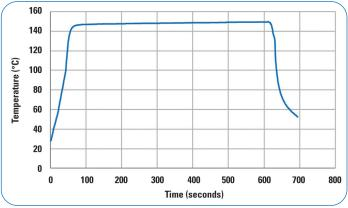
Figure 4. Drying profile: 10 minutes @ 150°C.
