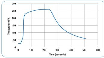
Figure 5. Sinter profile: 3 minutes, 250°C @ 20MPa.
