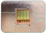
Figure 5. Die bonded on AMB substrate.
