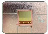
Figure 5. Die bonded on AMB substrate.
