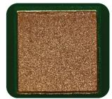
Figure 3. Printed paste deposit.
