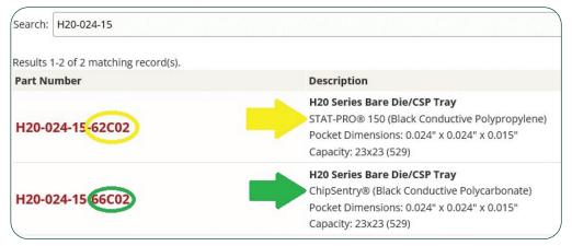
The material of the waffle tray is also embossed on the waffle tray, just like the part number is. In this case, it is ChipSentry<sup>®</sup>, which corresponds to the part number with the 66C02 suffix. Click on the correct part number.
