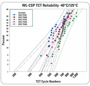
As shown in the Weibull plot for TCT reliability, Durafuse® LT can lead to an improvement over SAC305 over a wide range of peak temperatures. Durafuse® LT can also yield an improvement in drop shock reliability over SAC305.
