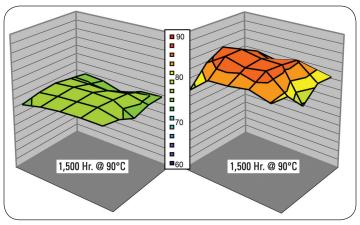
*Figure 8. Temperature profiles of TIM materials after thermal exposure. The bake-out profile of grease is shown on the right in contrast to a stable metal TIM on the left.*
