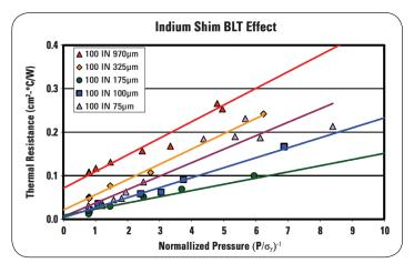
*Figure 5. Plot showing the relationship thermal resistance vs. the inverse of pressure.*
