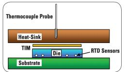
Figure 2. Schematic of TIM thermal test vehicle.
