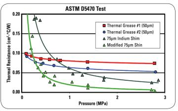
Figure 3. Plot of the thermal resistance of several TIM materials as a function of applied clamping pressure.
