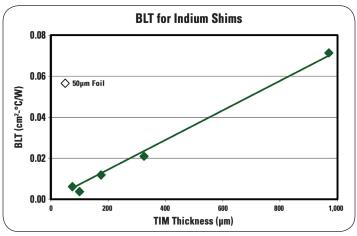
*Figure 6. BLT thermal resistance contribution for the indium metal TIM.* peak in this area develops and grows with time.
