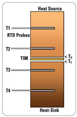
*Figure 1. Schematic of TIM and test block configuration of ASTM D5470 tester.*
