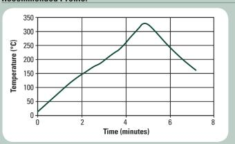
This profile is for use with Indalloy®151 (92.5Pb/5.0Sn/2.5Ag) and Sn10 (88Pb/10Sn/2Ag) alloys and will serve as a general guideline in establishing a reflow profile for your process. Adjustments will be necessary for use with other alloys. Various board geometries, densities, and oven types may require further profile adjustments.
