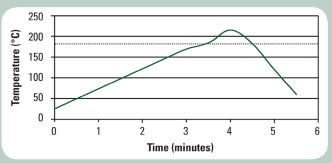
This reflow profile is designed for use with Sn63/Pb37 and Sn62/Pb36/Ag2 alloys. It will serve as a general guideline in establishing a reflow profile for this process. Adjustments to this profile may be necessary based on specific process requirements and the use of alloys with different melting temperatures.
