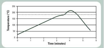
Peak reflow temperature should be <340°C in an air or nitrogen atmosphere (<100ppm  $O_2$ ), with a linear ramp up to 30°C above liquidus temperature. These profiles are recommended to the user as starting points, and should be optimized by the user to meet their individual process needs.
