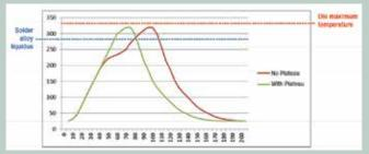
The diagram provides two examples of acceptable reflow profiles for use with 80Au/20Sn solder alloy and a maximum allowed die temperature of 325°C. General reflow guidelines for other solders are below.
