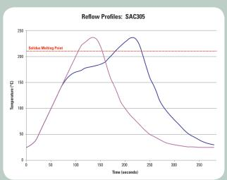
A short preheat (150–160°C) for less than 45 seconds may be used to reduce voiding. The profile should ideally be a linear ramp at 1–2°C/second up to 20–30°C above solidus temperature, with a rapid cool down afterwards, and a minimum time above liquidus of 20 seconds.
