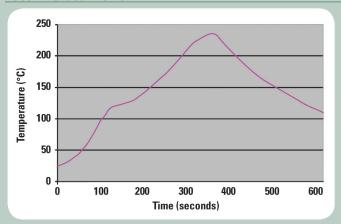
Flip-Chip Flux NC-826 is intended to be used in a nitrogen reflow environment of 100ppm oxygen or less. Some applications can utilize this material in an air environment, although best results will be obtained in an inert atmosphere. Flip-Chip Flux NC-826 can be used on many surface finishes including immersion Ag, Cu, and AuNi. These surfaces can be soldered with Pb-free alloys, but require nitrogen if reflow temperatures exceed 240°C.
