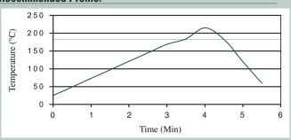
The profile shown here is designed for **Indium6.2** with Sn63/Pb37 and Sn62/Pb36/Ag2 under both air and nitrogen reflow atmospheres. It serves as a general guideline in establishing a reflow profile for these alloys.
