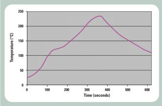
**TACFlux®10-ULR** is intended to be used in a nitrogen reflow environment of 100ppm oxygen or less. Some applications can utilize this material in an air environment, although best results will be obtained in an inert atmosphere. **TACFlux®10-ULR** can be used on many surface finishes including immersion Ag, Cu, and AuNi. These surfaces can be soldered with Pb-free alloys, but require nitrogen if reflow temperatures exceed 240°C.
