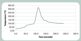
The typical profile above is designed for use with Sn10/Pb88/Ag2 or Sn5/Pb92.5/Ag2.5 alloy in a nitrogen atmosphere (500ppm oxygen or less). It can serve as a general guideline for establishing a profile for your process and should be regarded as a typical example. Adjustments to this profile may be necessary based on assembly size, thermal density, and other factors. Use of other alloys with lower or higher liquidus temperatures will also require changes.
