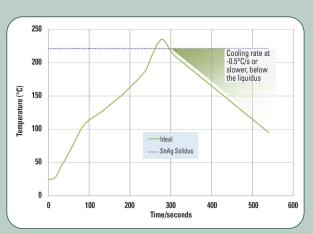
Profile optimized for thin die/thin substrate flip-chip.
