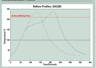
A short preheat (150–160°C) for less than 45 seconds may be used to reduce voiding. The profile should ideally be a linear ramp at 1–2°C/second up to 20–30°C above solidus temperature, with a rapid cool down afterward, and a minimum time above liquidus of 20 seconds.
