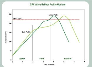
The stated profile recommendations apply to most Pb-free alloys in the SnAgCu (SAC) alloy system, including SAC305 (96.5Sn/3.0Ag/0.5Cu). This can be used as a general guideline in establishing a reflow profile when using **Indium9.0E** solder paste. Deviations from these recommendations are acceptable, and may be necessary, based on specific process requirements, including board size, thickness, and density.
