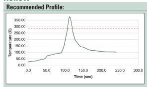
The typical profile above is designed for use with high-Pb (lead content 80% or greater) alloys in a forming gas or nitrogen atmosphere (100 ppm oxygen or less). This profile can serve as a general guideline for establishing a profile for your process and should be regarded as a typical example. Adjustments to this profile may be necessary based on assembly size, thermal density, and other factors. Use of other alloys with lower or higher liquidus temperatures will also require changes.
