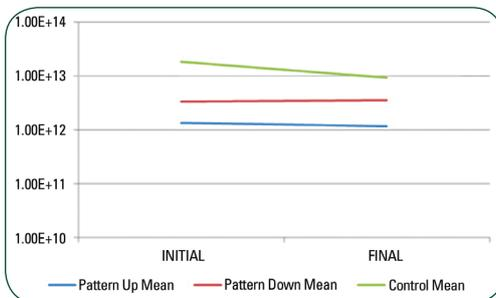
The electromigration test is performed to IPC-TM-650 method 2.6.14.1 with boards prepared using IPC-TM-650 method 2.6.3.3. The test conditions for this test are 496 hours at  $65^\circ\text{C} \pm 2^\circ\text{C}$  and  $88.5\% \pm 3.5\%$  RH. To pass this test, there should be no visible corrosion and no dendritic growth that decreases line
