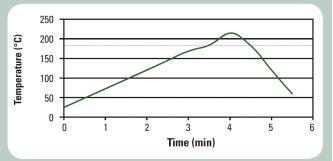
Peak reflow temperature should be <350°C in an air or nitrogen atmosphere (<500ppm  $O_2$ ), with a linear ramp up to 30°C above liquidus temperature. These profiles are recommended to the user as starting points, and should be optimized by the user to meet their individual process needs.
