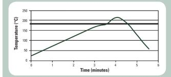
Peak reflow temperature should be <340°C in a nitrogen atmosphere (<100ppm  $O_2$ ), with a linear ramp up to 30°C above liquidus temperature. These profiles are recommended to the user as starting points, and should be optimized by the user to meet their individual process needs.
