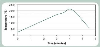
This profile is designed for use with Indalloy<sup>®</sup>205 (60ln/40Pb) MP 181°C and Indalloy<sup>®</sup>227 (77.2Sn/20ln/2.8Ag) MP 187°C. It will serve as a general guideline in establishing a reflow profile for your process. Adjustments to this profile may be necessary based on specific process requirements and the use of alloys with different melting temperatures.
