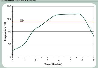
This profile is designed for use with Indalloy®281 and can serve as a general guideline in establishing a reflow profile for use with other alloys. Adjustments to this profile may be necessary based on specific process requirements.
