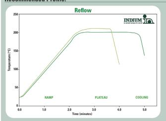
This profile is designed for use with Durafuse® LT in Indium5.7LT-1. This can be used as a general guideline in establishing a reflow profile for **Durafuse® LT** Solder Paste. Deviations from these recommendations are acceptable, and may be necessary, based on specific process requirements.
