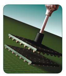
is being used in the dipping process. The settings will depend upon the package bump height and pitch. Other equipment settings can also have an effect on the process including the flux shear speed, insertion speed, and extraction speed.
