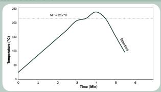
**SiPaste® 3.2HF** should be reflowed using a linear profile in an air or nitrogen atmosphere. The stated profile recommendations can be used as a general guideline in establishing a reflow profile for **SiPaste® 3.2HF** with SnAgCu, SnAg, and SnSb alloy systems.
