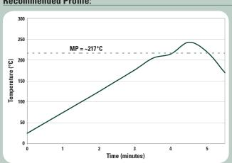
The above reflow profile was designed to serve as a starting point for process optimization using Indium3.1 Solder Paste. When seeking to minimize thermal gradient or reduce voiding in BGA assemblies, a profile utilizing a soak of up to 2 minutes at 205–210°C may help.
