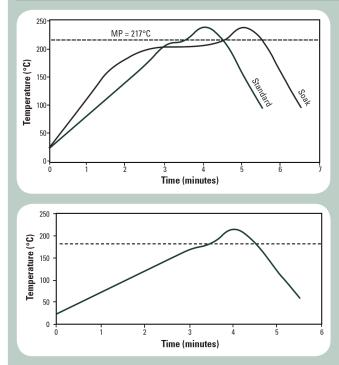
Peak reflow temperature should be <350°C in an air or nitrogen atmosphere (<500ppm  $O_2$ ), with a linear ramp up to 30°C above liquidus temperature. These profiles are recommended to the user as starting points, and should be optimized by the user to meet their individual process needs.
