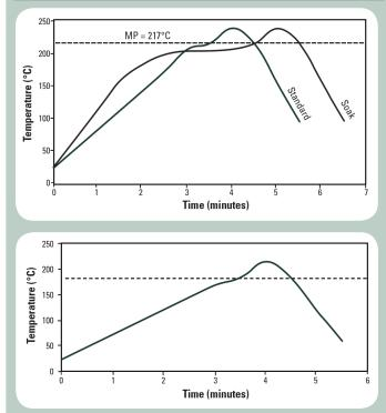
Peak reflow temperature should be  $<350^{\circ}$ C in an air or nitrogen atmosphere (<500ppm O<sub>2</sub>), with a linear ramp up to 30°C above liquidus temperature. These profiles are recommended to the user as starting points, and should be optimized by the user to meet their individual process needs.
