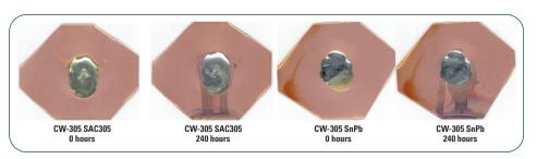
since the residue from this flux is designed to be removed with water and should not be left on the board for 240 hours, this reaction product should not be a concern.
