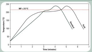
The stated profile recommendations apply to most Pb-free alloys in the SnAgCu (SAC) alloy system, including SAC305 (96.5Sn/3.0Ag/0.5Cu). This can be used as a general guideline in establishing a reflow profile when using **Indium5.1** Solder Paste. Deviations from these recommendations are acceptable, and may be necessary, based on specific process requirements, including board size, thickness, and density.
