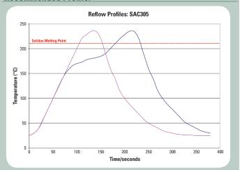
A short preheat (150–160°C) for less than 45 seconds may be used to reduce voiding. The profile should ideally be a linear ramp at 1-2°C/second up to 20-30°C above solidus temperature, with a rapid cool down afterwards, and a minimum time above liquidus of 20 seconds.
