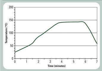
Peak reflow temperature should be close to  $150^{\circ}$ C in a nitrogen atmosphere (<100ppm  $0_2$ ), with a linear ramp up to  $30^{\circ}$ C above liquidus temperature. These profiles are recommended to the user as starting points, and should be optimized by the user to meet their individual process needs.
