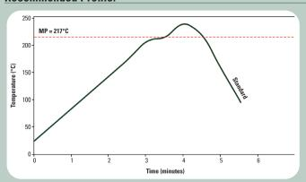
Indium3.2HFA should be reflowed using a linear profile in an air or nitrogen atmosphere. The stated profile recommendations can be used as a general guideline in establishing a reflow profile for Indium3.2HFA with SnAgCu alloy systems.
