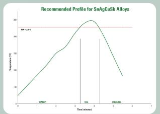
The stated profile recommendations apply to most Pb-free alloys in the SnAgCu (SAC) alloy system, including SAC305 and SnAgCuSb.This can be used as a general guideline in establishing a reflow profile when using **Indium8.9HFRV Solder Paste**. Deviations from these recommendations are acceptable, and may be necessary, based on specific process requirements, including board size, thickness, and density. Start with the linear profile, then move to the optional soak profile, if needed.
