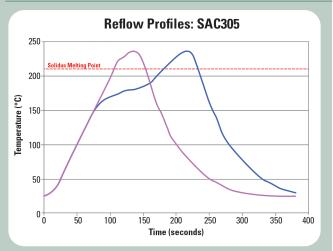
**NC-809 Flux** is intended to be used in a nitrogen reflow environment of 100ppm oxygen or less. Some applications can utilize this material in an air environment, although best results will be obtained in an inert atmosphere.
