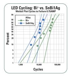
Bi+ samples in the chart (left) demonstrated improved reliability when experiencing LED power cycling versus standard Bi-based alloys.
