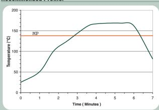
This profile is designed for use with Bi+ with **Indium5.7LT-1**. This can be used as a general guideline in establishing a reflow profile for Bi+ solder paste. Deviations from these recommendations are acceptable and may be necessary, based on specific process requirements.
