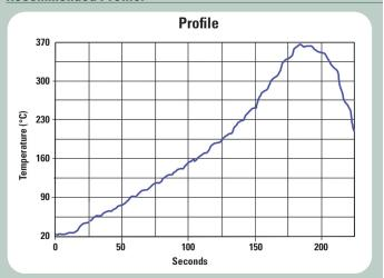
The profile above is designed for use with **Durafuse® HT** in a nitrogen atmosphere or forming gas (<100ppm  $0_2$ ). Recommended peak temperature is 350–385°C. It can serve as a general guideline for establishing a profile for your process and should be regarded as a typical example. Adjustments to this profile may be necessary based on assembly size, thermal density, and other factors.
