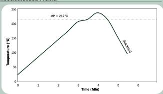
Indium6.6HF-HD should be reflowed using a linear profile in an air or nitrogen atmosphere. The stated profile recommendations can be used as a general guideline in establishing a reflow profile for Indium6.6HF-HD with SnAgCu, SnAg, and SnSb alloy systems.
