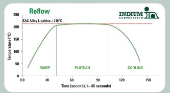
This profile is designed for use with Indium5.7LT-1 with Indalloy®301. This can be used as a general guideline in establishing a reflow profile for Indium5.7LT-1 Solder Paste. Deviations from these recommendations are acceptable, and may be necessary, based on specific process requirements.
