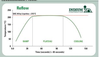
This profile is designed for use with Indium5.7LT-1 with Indalloy®301. This can be used as a general guideline in establishing a reflow profile for Indium5.7LT-1 Solder Paste. Deviations from these recommendations are acceptable, and may be necessary, based on specific process requirements.
