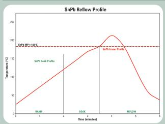
Start with the linear profile, then move to the optional soak profile, if needed.
