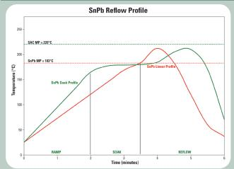
This profile is designed for use with Sn63/Pb37 and Sn62/Pb36/ Ag2 and can serve as a general guideline in establishing a reflow profile for use with other alloys. Adjustments to this profile may be necessary based on specific process requirements. Start with the linear profile, then move to the optional soak profile, if needed.
