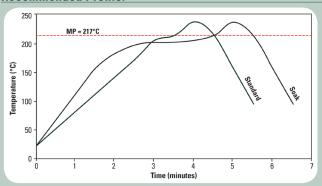
The stated profile recommendations apply to most Pb-free alloys in the SnAgCu (SAC) alloy system, including SAC305 (96.5Sn/3.0Ag/0.5Cu). This can be used as a general guideline in establishing a reflow profile when using **Indium5.1AT** Solder Paste. Deviations from these recommendations are acceptable, and may be necessary, based on specific process requirements, including board size, thickness, and density.
