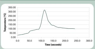
The typical profile above is designed for use with Sn10/Pb88/Ag2 or Sn5/Pb92.5/Ag2.5 alloy in a nitrogen atmosphere (500ppm oxygen or less). It can serve as a general guideline for establishing a profile for your process and should be regarded as a typical example. Adjustments to this profile may be necessary based on assembly size, thermal density, and other factors. Use of other alloys with lower or higher liquidus temperatures will also require changes.
