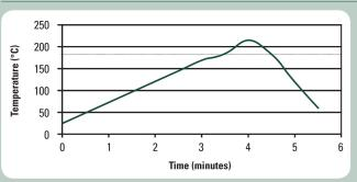
The profile shown here is designed for Indium6.3 with Sn63/Pb37 and Sn62/Pb36/Ag2 under both air and nitrogen reflow atmosphere. It serves as a general guideline in establishing a reflow profile for these alloys.
