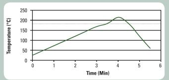
Peak reflow temperature should be <260°C in an air or nitrogen atmosphere (<500ppm  $O_2$ ), with a linear ramp up to 30°C above liquidus temperature. These profiles are recommended to the user as starting points, and should be optimized by the user to meet their individual process needs.
